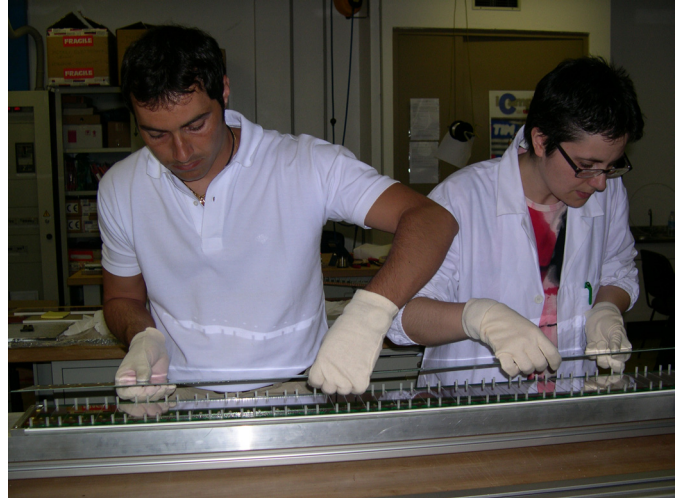
Fig. 6. Photographs of the MRPC during the assembly. The upper picture shows an open MRPC strip. The lower picture shows the positioning of the central PCB, with two external glasses glued on both sides of it
