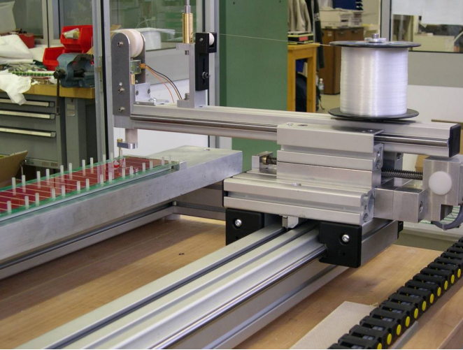
Fig. 5. Photograph of the first prototype of fishing-line stretching machine
